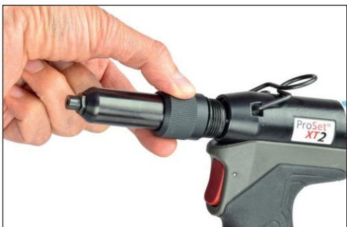
Quick disconnect nose housing and jaw case (without tools)
