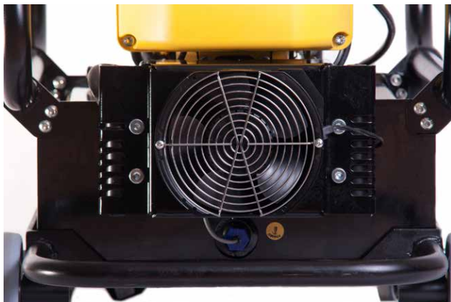
Reservoir heat exchanger
